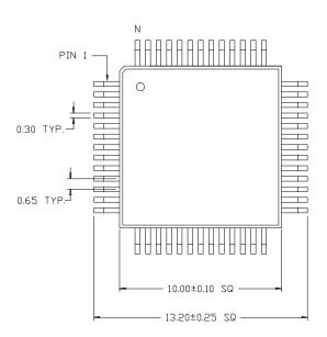
DIMENSIONS ARE IN MILLIMETERS LEAD COPLANARITY 0.102 MAX.
